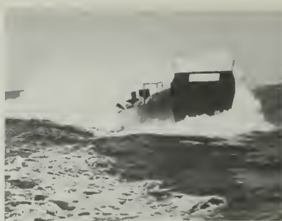
SMOKER —Navy landing craft lays down a smoke screen with a gas turbine used as a smoke generator.
